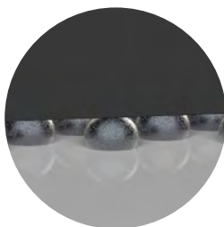
BGA attach to board for greater density and optimized trace breakout region
