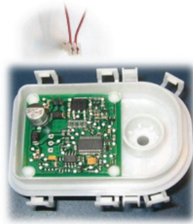
Control for urea injection
